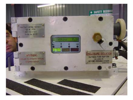
Manufacturer :- Nautitech Mining Services Dimensions :- 350 (L) x 200 (H) x 155 (D) Weight :- 37kg
